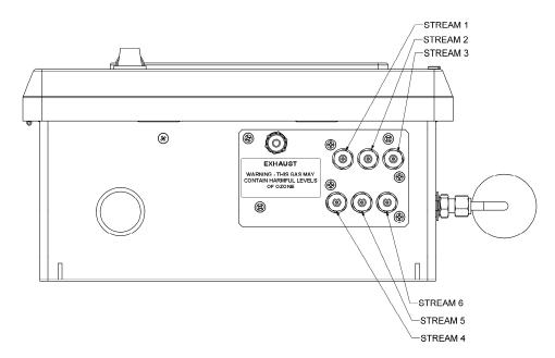
Figure 4-4: Pneumatic Connections, NEMA Configuration, Multi-Stream
